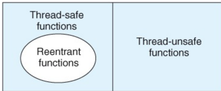
Figure 12.39 Relationships between the sets of reentrant, thread-safe, and thread-unsafe functions.
